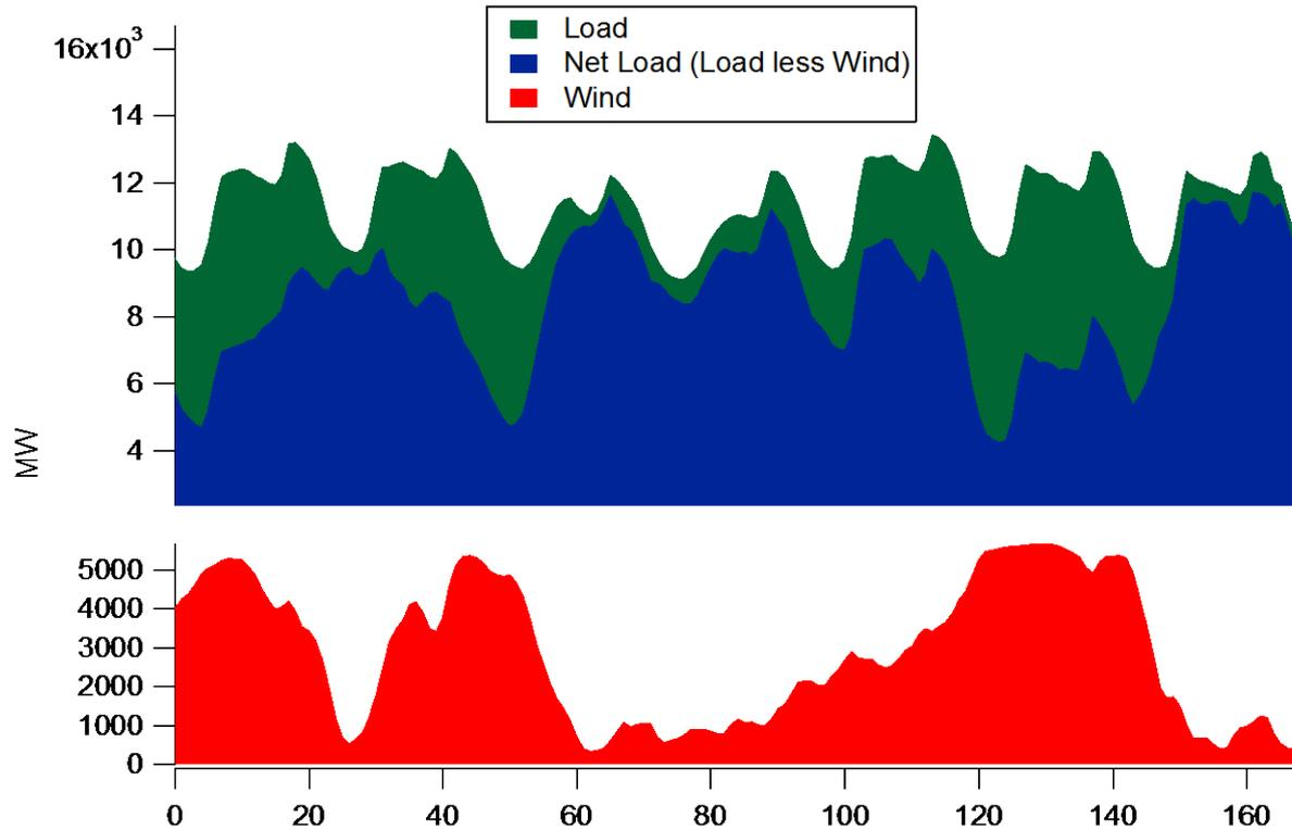
Steeper ramps and lower turndown levels in some cases (top) are examples of the increased flexibility required by systems with large amounts of wind energy.
